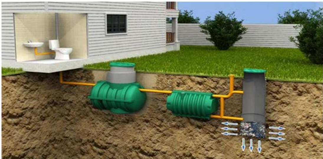
Figure 5.1 - Space-efficient septic tank system for residential use
